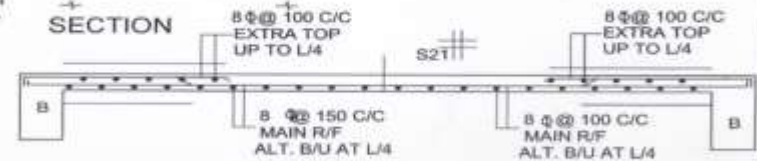
SLAB DETAILS AT "B-B"
